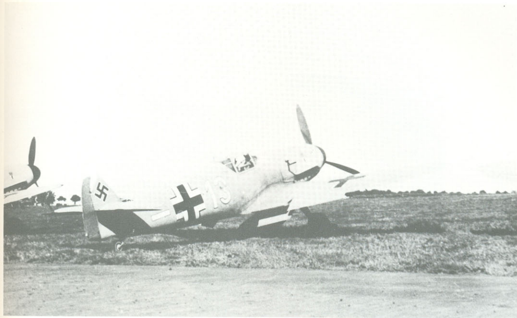
Upper. This Bf 109F, White 13 of 4./JG 27, like the aircraft on each side of it, had considerably faded paintwork, almost certainly tan 79 upper surfaces over 78 sky blue. Continuous desert operations produced an effect on aircraft finishes not unlike the effect of energetically applied sandpaper. Lower. Two derelict but interestingly marked Bf 109Fs of III./JG 27 discovered by Australian forces in North Africa after the German retreat. Both show the standard 78/79 scheme and white markings.
