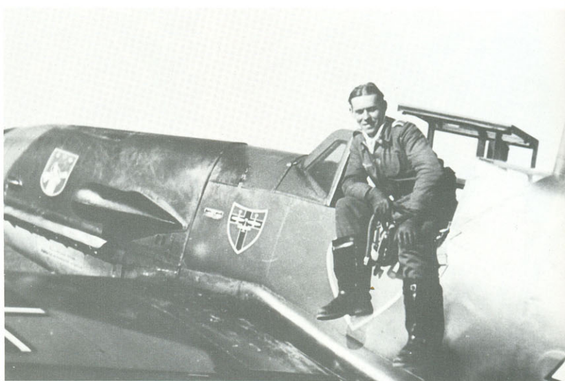
Left and lower. Two informal shots of Fw Halfmann in front of his Bf 109G, White 7, which carried three-tone camouflage on the upper surfaces. These colors can best be described as a light tan (seen near the nose), a medium green a little darker than RLM 83, and a very dark olive green similar to RLM 70. Many other aircraft of the unit utilised the same basic scheme.
